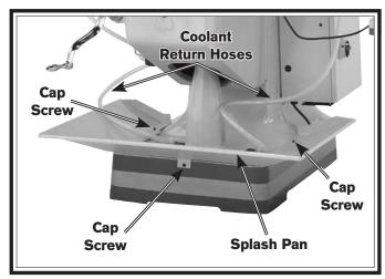
Figure 12. Splash pan and coolant return hoses installed.
